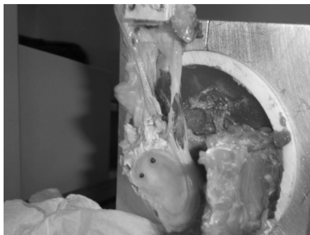
Figure 5. Capsular tissue failure after pull-to-failure testing.
